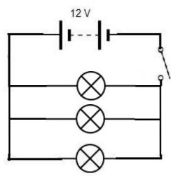
side and rear lamps in parallel with headlamp; side and rear lamps in parallel with each other;
